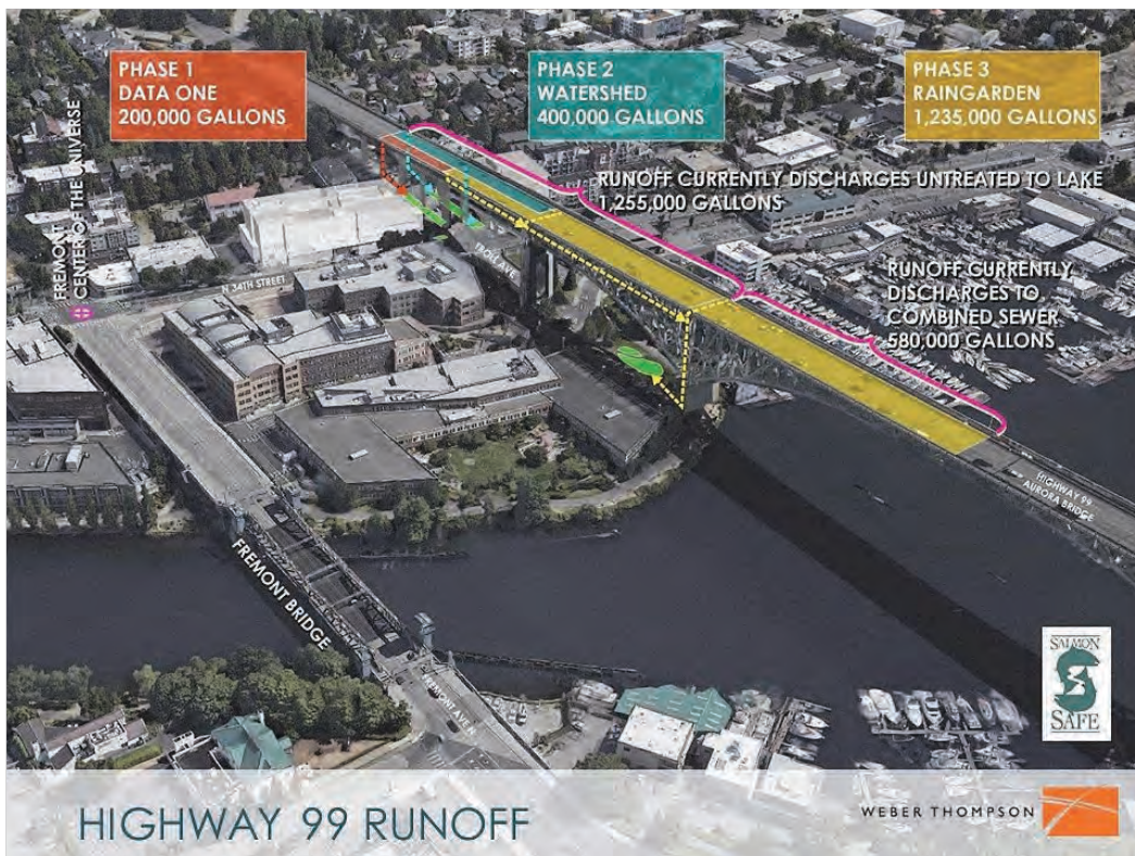
This bridge aerial illustration shows where the bridge downspouts and mitigation project are located and where runoff will be contained and treated through bioswales.
